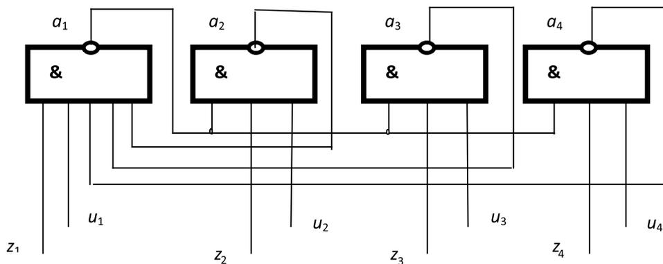
Fig. 1. MFIS class L on the elements of the AND-NOT
