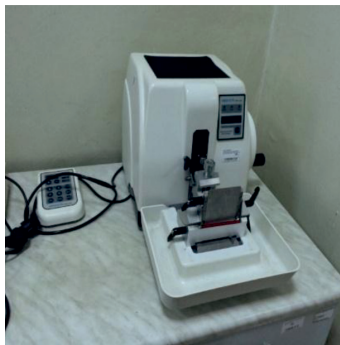
a) Semi-automatic microtome HEOTION ERM 3100 for the preparation of ultra-thin sections
