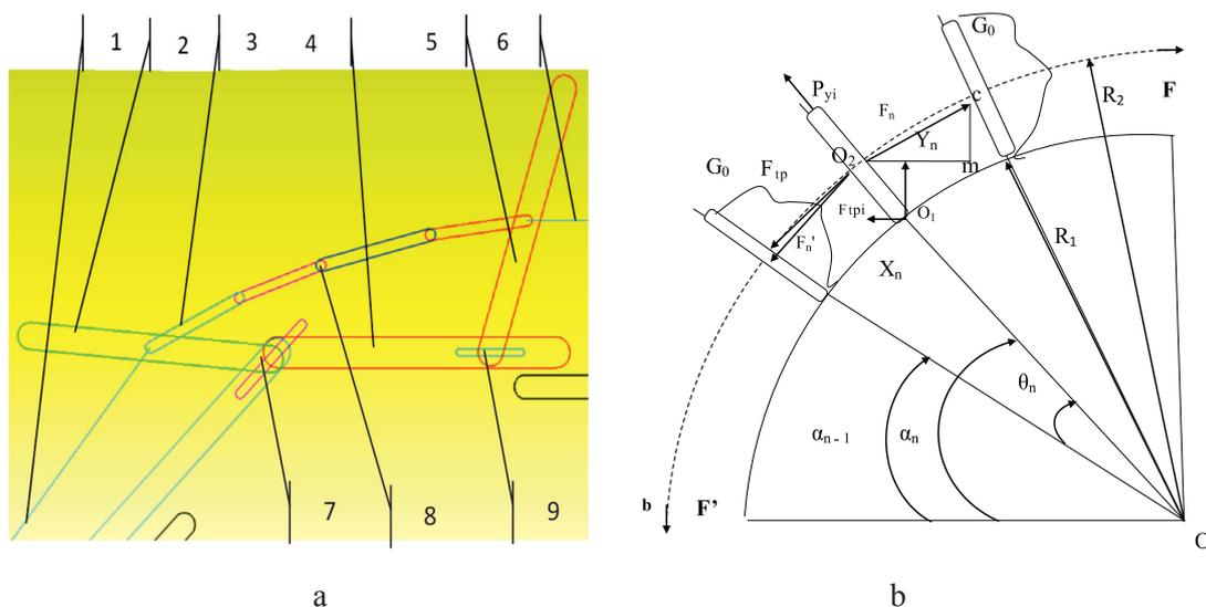
Fig. 1. Location of the scrapers and the chain links and their movement (a); an idealized diagram of loading on the rotary troughs (b): 1,6 – tractive forces direction; 2,5 – scrapers in the end of the run; 3 – the chain links; 4 – troughs; 7,8 – hinges in the bottom and top troughs, 8 – spherical hinge of the chain central link
