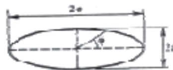
Fig. 2. The scheme of the elliptical-shaped crack
