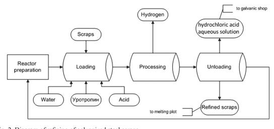
Fig. 2. Diagram of refining of galvanized steel scraps
