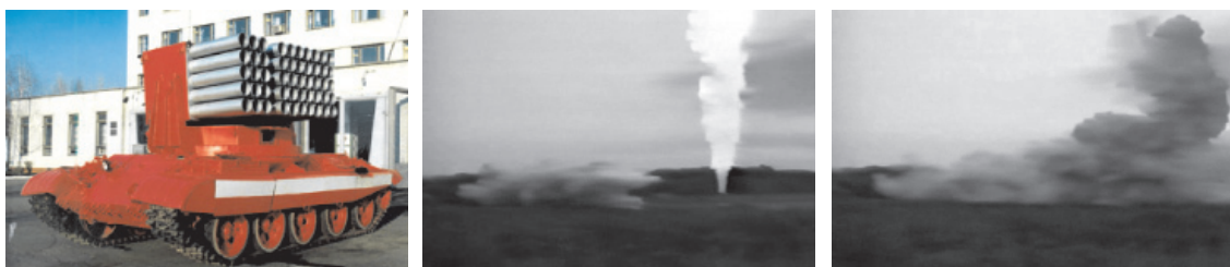
Fig. 2. “Impulse-3M” system with 50-barreled turret MM installed onto the armored chassis of T-62 tank. Each barrel contains up to 20–25 kg of the working mixture. The MM working distance is up to 120 m, the area covered by the only volley is up to 3500 square meters. This “Impulse-3M” can extinguish the gas well with reservoir pressure 140 atm and gas expence 1,2 million cubic meters per 24 hours at one second by the volley from its 10 barrels
