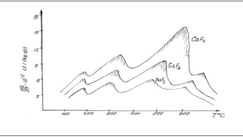
The Drawing one shows the velocity dependency of emitting the accumulated energy on the temperature for crystals  $CaF_2$ ,  $S\tau F_2$ ,  $BaF_2$  which are irradiated by the identical absorbed dose of  $\gamma$ -ray. The areas limited by curved  $\frac{dQ}{dT}$  determine the radiation energy accumulated by crystals.
