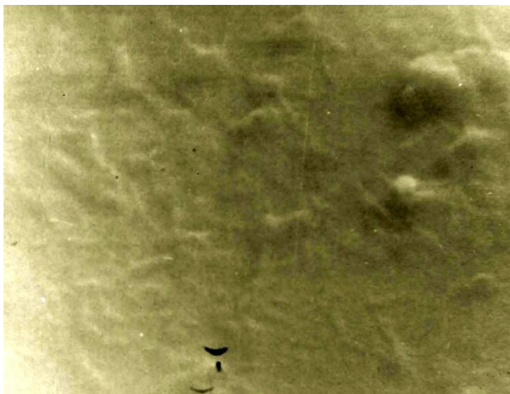
Figure 4. Morphology of the prism \{001\} face formed by intergrowth of separate needles (x6000).
